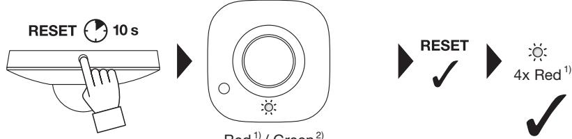
Release button devices perform reset action, after devices return to factory default.<sup>3)</sup>
