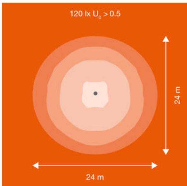
Floodlight Max 900W SYM 60 simplified isolux diagram
