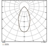
SP CBO FIX V 6W 930 CPS DIM 60DEG IP65WT 580lm
