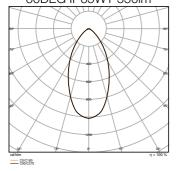
SP CBO FIX V 6W 927 CPS DIM 60DEG IP65WT 550lm
