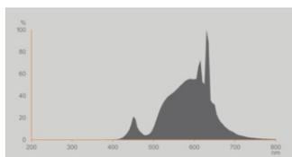
EPREL Data Spectral Diagram LEDr
