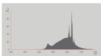
EPREL Data Spectral Diagram LEDr
