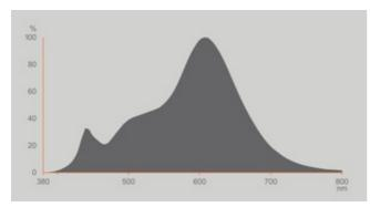
EPREL Data Spectral Diagram LEDr\_Stick 2700K\_927
