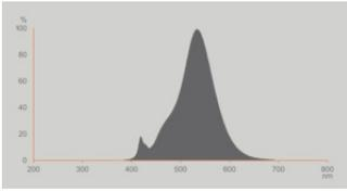
EPREL Data Spectral Diagram LEDr
