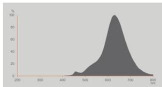
EPREL Data Spectral Diagram LEDr
