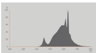
EPREL Data Spectral Diagram LEDr
