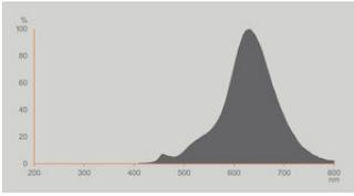
EPREL Data Spectral Diagram LEDr
