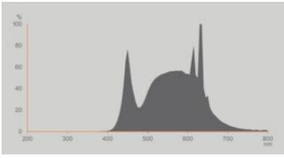
EPREL Data Spectral Diagram LEDr
