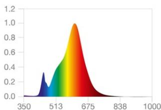
EPREL Data Spectral Diagram LEDr
