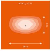
Streetlight Flex 80W RV25ST simplified isolux diagram
