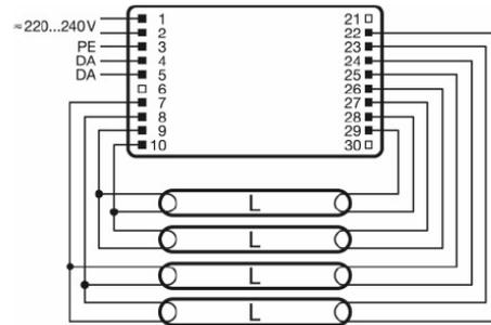
Max. permitted cable length between ECG and lamp: 1,0 m
