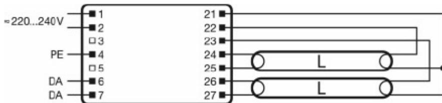
Max. permitted cable length between ECG and lamp: 1,5 m (PIN 21; 22), 1,0 m (PIN 24; 25; 26; 27)
