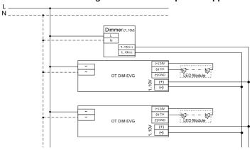
Control of more OT 80/220-240/24 DIM P to an external Dimmer/Potentiometer. Thanks to the fully isolated 1...10V interface, two different kind of dimming devices are possible
