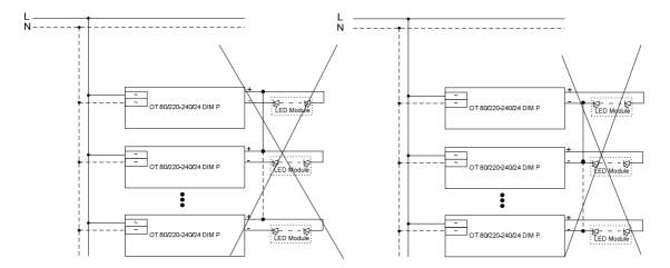
a) The installation of two ore more OPTOTRONIC® OT 80/220-240/24 DIM P Power supplies with common "-" or "+" is forbidden.
