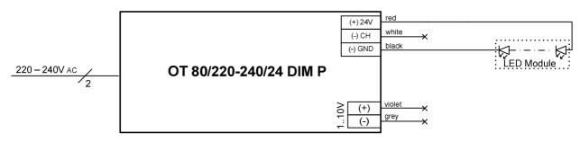
Ensure proper insulation of not connected wire terminals.
