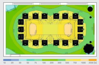
Isolux lines indicate the light levels reached at all surfaces of a room. This is to make sure that the light planning complies with norms of e.g. Em>500 Ix at desk surfaces.
