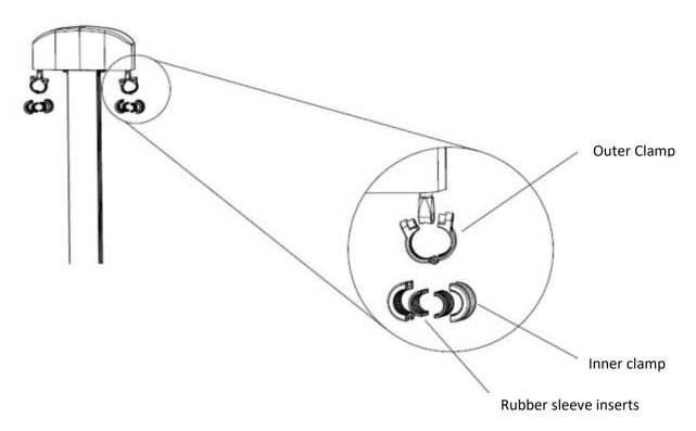
4. Use the correct size rubber sleeve inserts and attach them to the charging cable with the inner clamp. Adjust the charging cable such that it is above the ground when the cable management system is fully retracted. Lock the charging cable in place with the (4) M3 screws provided. Reattach the outer clamp.
