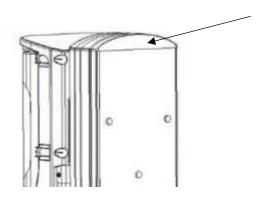
2. Next, insert the pedestal extender into the base pedestal and use the 4 included M5 screws to secure the pedestal extender into place.
