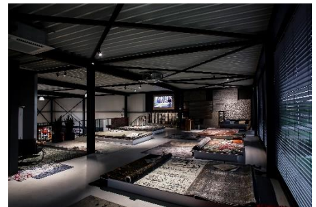
LEDVANCE TRACKLIGHT SPOT luminaires were used for general but also for accent lighting.
