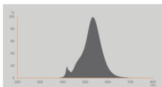
EPREL Data Spectral Diagram LEDr
